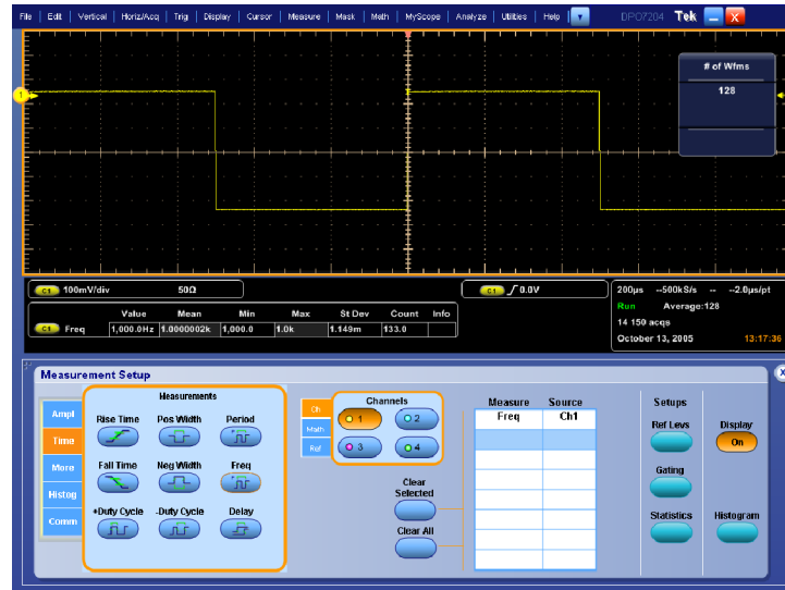
Figure 2-29: Measurement of probe compensator frequency
